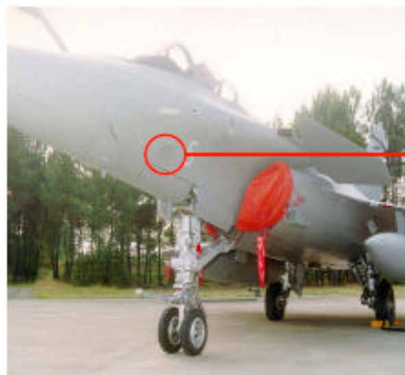
3a, 3b INTEGRATED LADDER CONTROL AND DEPLOYMENT SWITCH
