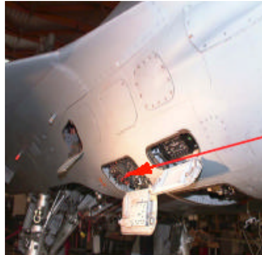
1a ENGINEER'S PANEL RIGHT SIDE
