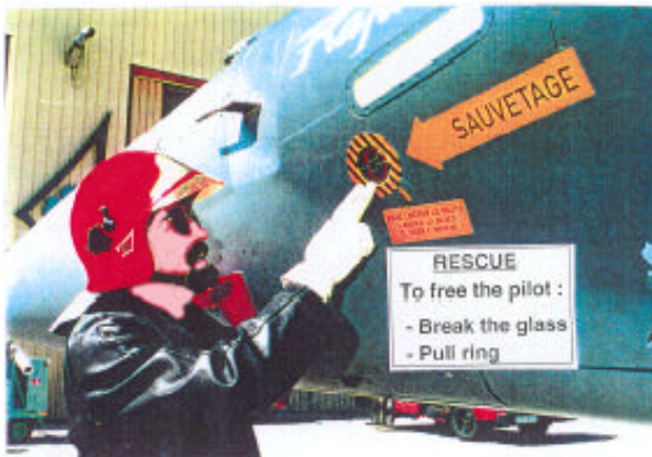
3a, 3b FRAGILIZATION PLEXIGLASS COVER (LH SHOWN) WITH ASSOCIATED PULL RING
