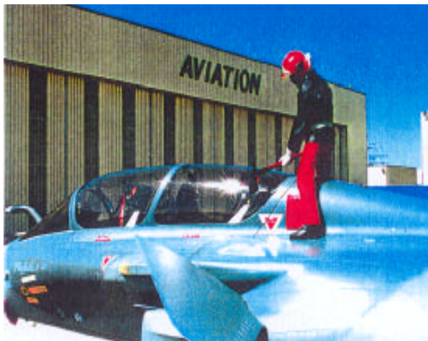
4b BREAKING CANOPY AT CENTRAL REAR
