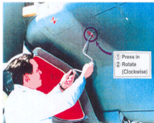
2h END PIECE ADAPTER 11 INSTALLED IN CANOPY CONTROL
