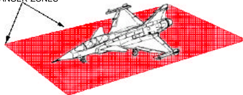
FRONT DANGER ZONE WITH ENGINE RUNNING 16.5 FT RADIUS
