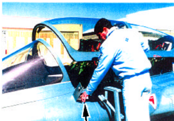
1a, 1b, 1c CANOPY CONTROL SWITCH AND DOOR
