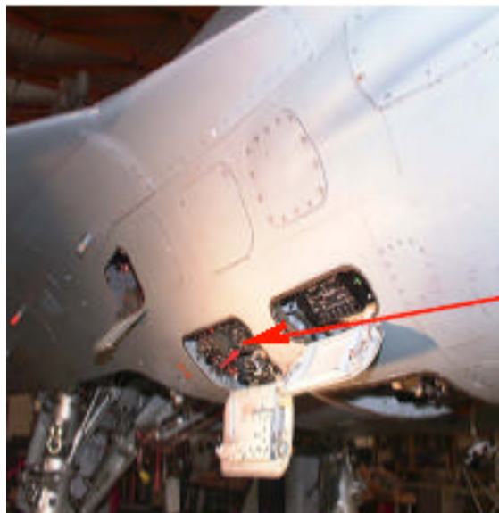
1a ARMAMENT SECURITY SWITCH
