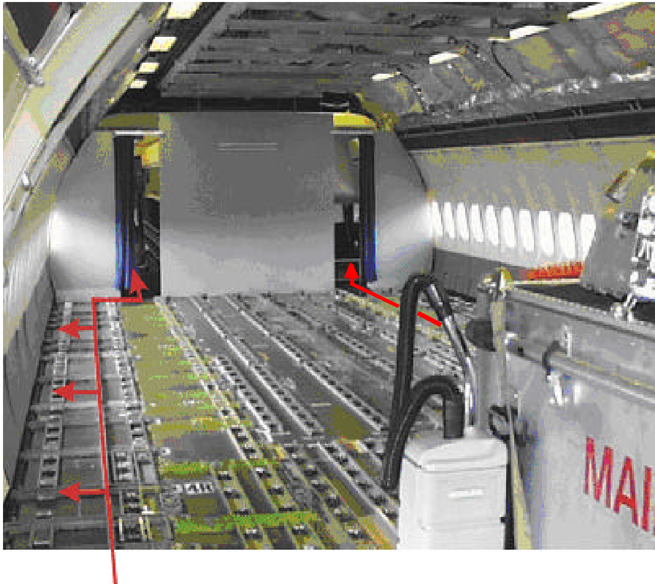
WALKING AREA AROUND CARGO PALLETS FOR ACCESSING PASSENGER COMPARTMENT (BOTH SIDES)
